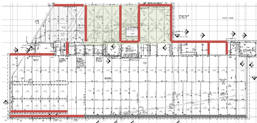
Figure 10: Level 5 Framing Plan Showing Lateral System (S-105) — Lateral Braced Frame — Gravity Truss that Contributes to Lateral System — Floor System with Diagonal Bracing
